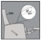
**Infinite Position Locking Back Lever**
